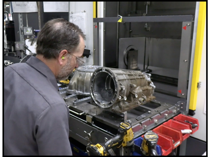
JASPER Associate Kyle Giesler removes a clean case and bellhousing from the Sugino CNC washer at the Power Drive facility.
