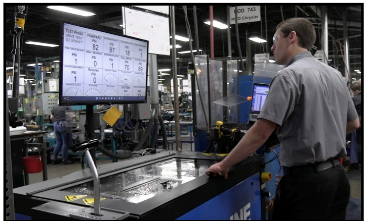
The Axiline VBT 8000 is used in valve body testing the Chrysler 46RE, 47RE and 48RE transmissions. Their popularity remains high due to their use in RAM diesel applications.
